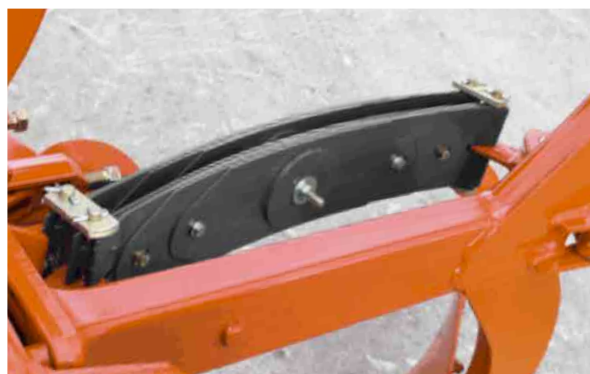
Montage double-pack : 14 lames (1400kg)
